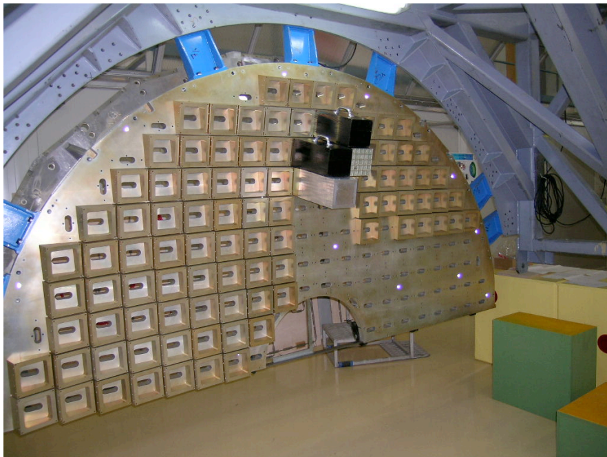
Figure CP 5: Submodules of the ECAL barrel in assembly jigs. Each submodule consists of 10 crystals in a glass-fibre alveola structure. Two APDs are glued to the rear of each crystal and the flexible kapton ribbons from the APDs, terminated with connectors, can be seen hanging down from the back of the submodules.
