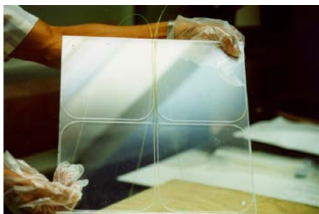
Figure 5.24: View of a typical tile of HO with WLS fibres inserted in the 4 grooves of the tile.
