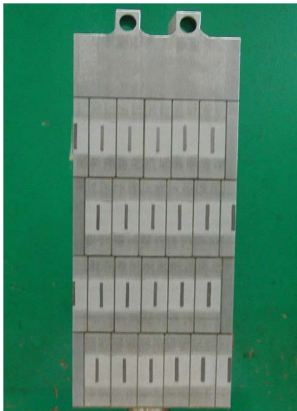
Figure 2.4: Cross section of the cold mass with the details of the 4-layer winding with reinforced conductor.
